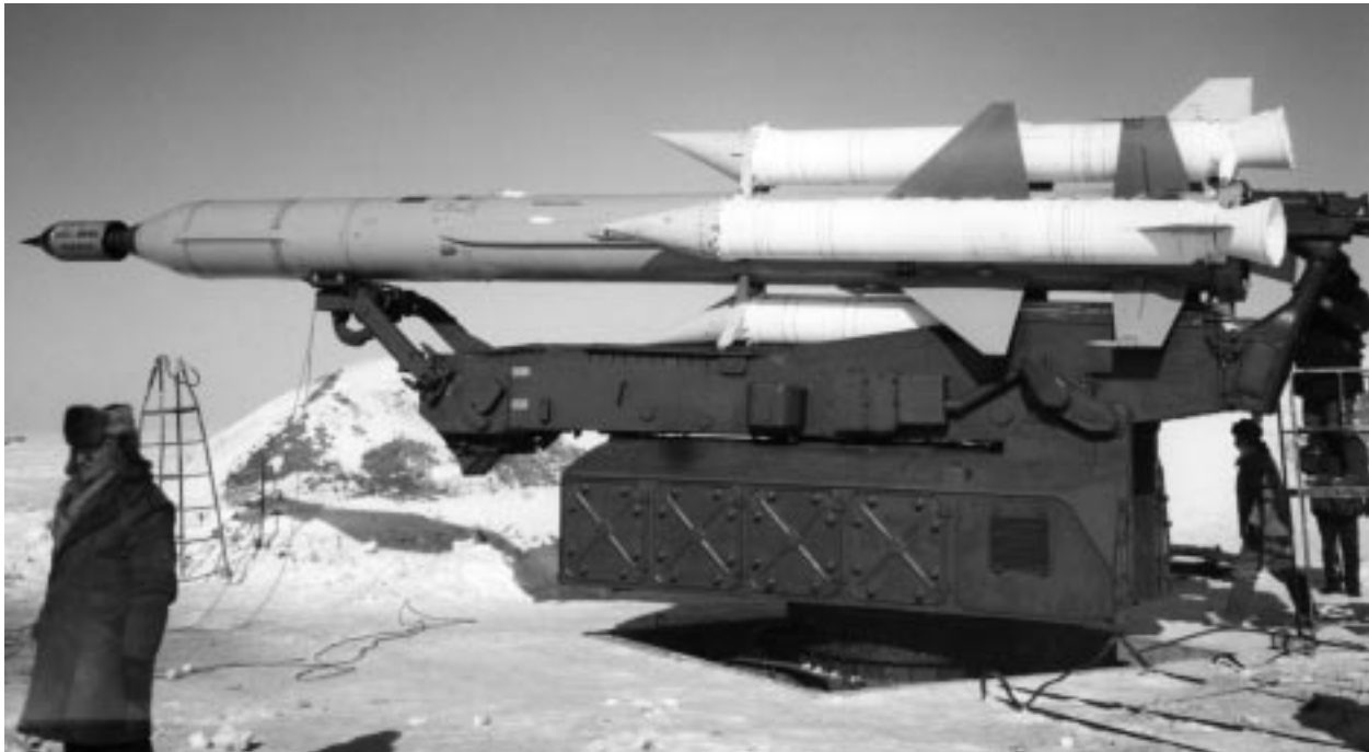
Figure 8. The SA-5 booster and HFL launch configuration.
