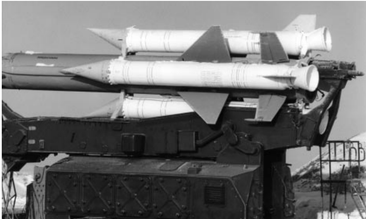
Figure 9. The SA-5 stabilization fin modification and strap-on boosters.
