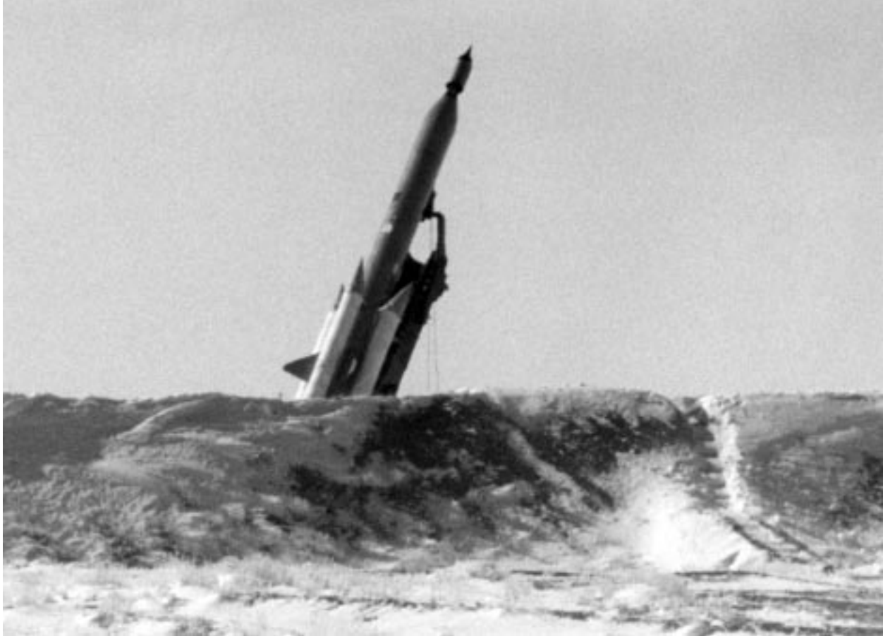
Figure 10. The SA5 configuration in the launch position.
